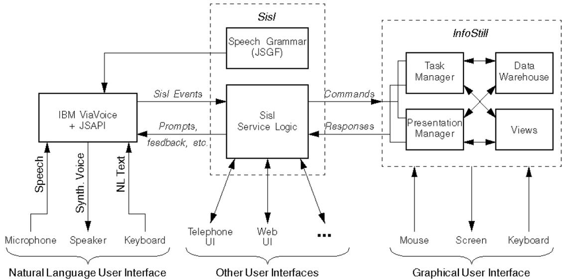
**Figure 2.** Overall System Architecture.
