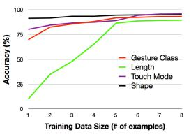
Figure 10. Improvement in average accuracy of gesture detection on the three surfaces with increasing size of training data.
