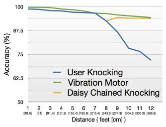
**Figure 7.** Performance of detecting devices on the same surface. User knocking performance drops significantly over larger distances, but this can be nullified using daisy chaining.
